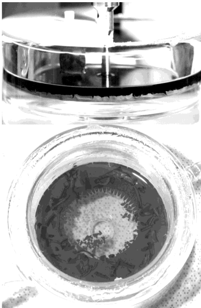
Figure 9. Top: View of the wrinkled film edge between the water and oil phases. The edge has extended into the oil phase and developed defects. Bottom: Film after oil removal. The large fragments resting on top of the film originated from the film edge, then extended upward into the oil phase, then fractured, and then fell off. The small triangular film pieces floating on top of the water phase were sheared off of the bulk film by the serrated bob edge.
